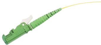
Integrated spring-loaded shutter for dust and scratching protection. Locking type latched push-pull. Injection-molded PBT housing, UL 94 V-0 (flammability index).
