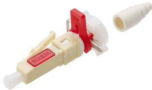
Field-terminable LC / PC connector, Grade Bmf/3, individual packaged incl. stripping chart and QR code with installation instructions. Color beige, strain relief pigtail white.
